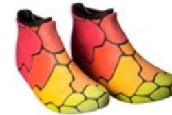
Shoes 3D printed on the Objet500 Connex3 Color Multi-material 3D Printer, in one print run, using Vero Yellow, VeroMagenta and rubber-like TangoBlack Plus
